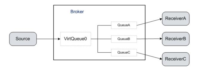
In this example, the broker has a virtual queue and three physical queues. The source sends messages to the virtual queue. The broker forwards the message to the physical queues. The receivers get messages from the physical queues.
