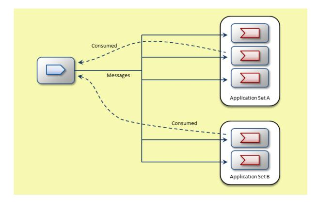
Subscribing applications create ULB receivers that register with a ULB source. The source adds each receiver to an application set according to a *receiver type ID* which is supplied by the subscribing application. The source's configuration defines which receivers are added to which application sets using the configuration option **umq\_ulb** $\leftarrow$  **\_application\_set (source)**.
