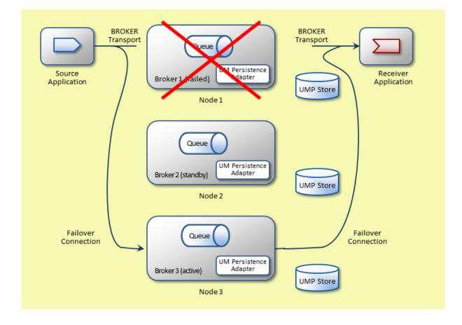
In this example, Broker1 has failed and disconnected from the client applications. The client applications then try all IP and port addresses on their broker option list until they find an open socket to connect to. If a client application does not find an active broker, it waits and then tries the list again. This cycle continues until the system elects a new active broker.
