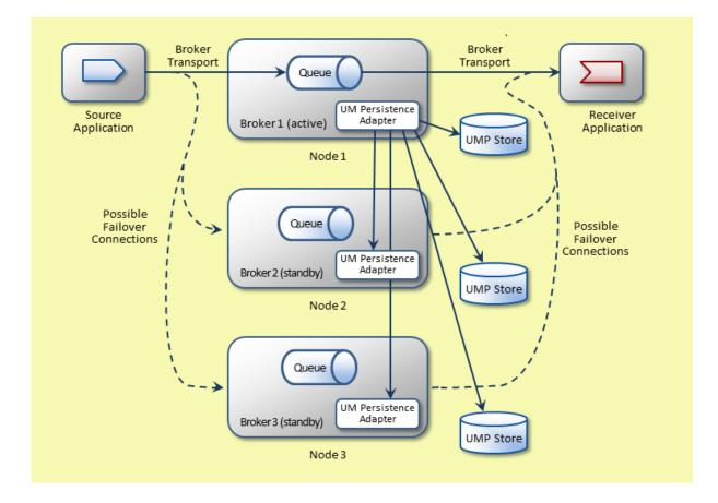
The source application sends a persistent message to the active broker. For each persistent message, the active broker performs the following operations:
