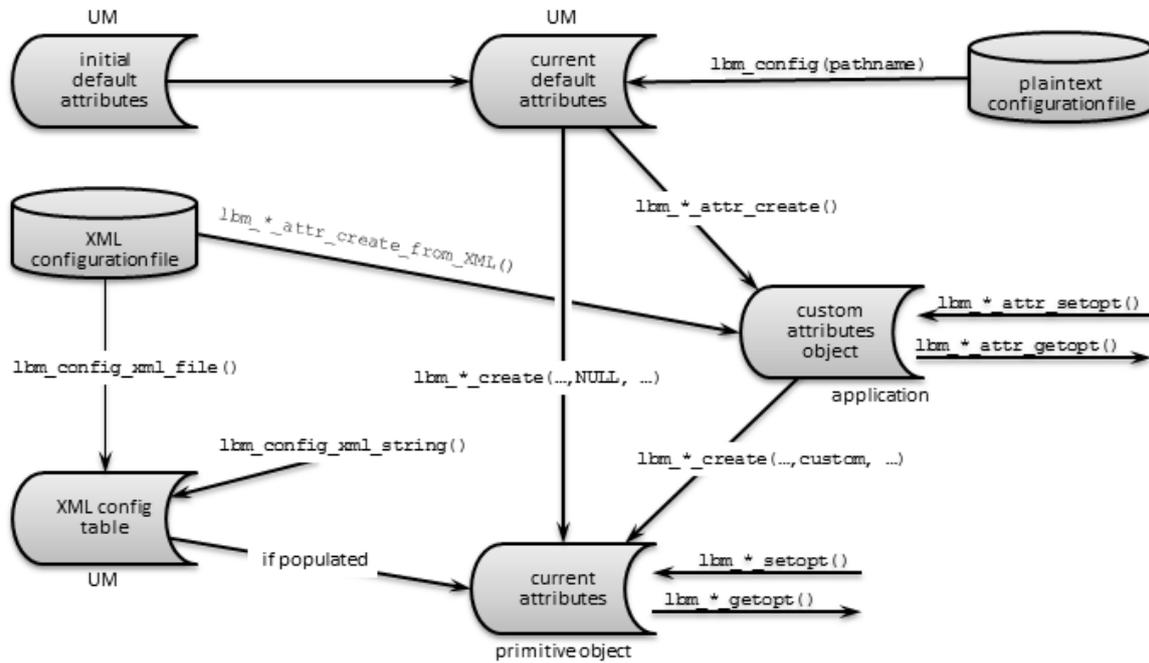
The *initial default attributes* is the set of factory defaults in Ultra Messaging. At process initialization time, these factory defaults are copied into a set of internal process-global attribute structures (*current default attributes*).
