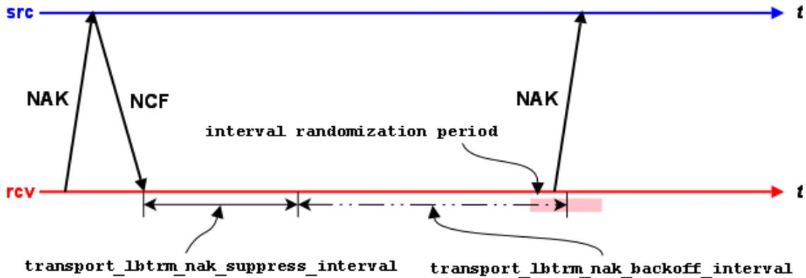
Following the receipt of an NCF, a receiver suppresses all NAK generation for that sequence number until `transport_lbtrm_nak_suppress_interval (receiver)` passes. NAK generation resumes with the usual `transport_lbtrm_nak_backoff_interval (receiver)` if repair was not received during the suppression interval.
