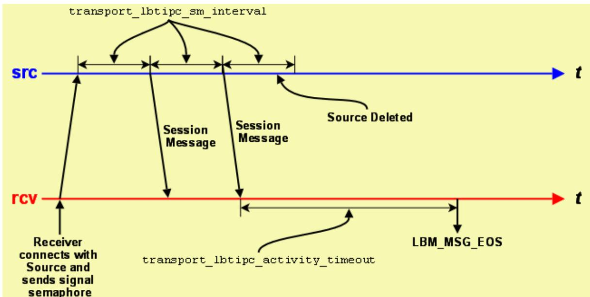
The Source Session Message mechanism enables the receiver to detect when a source goes away and works similarly to LBT-RU. It operates independently of message writes/reads in the Shared Memory Area.
