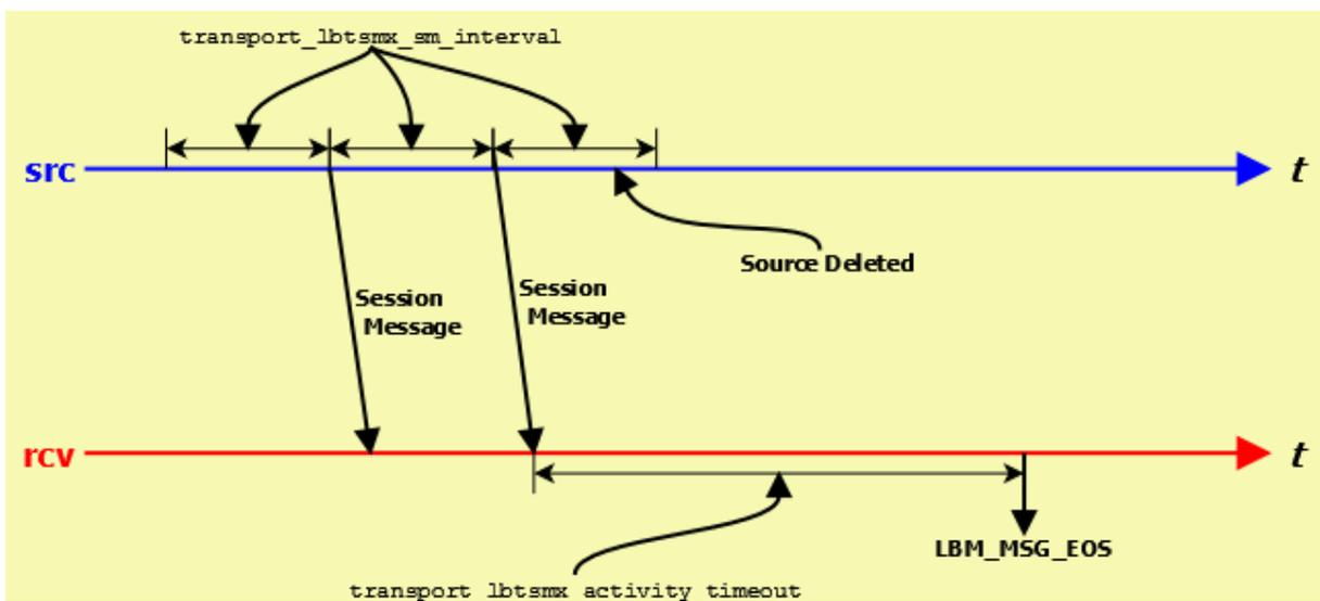
The Source Session Message mechanism enables the receiver to detect when a source goes away and works similarly to LBT-RU. It operates independently of message writes/reads in the Shared Memory Area.
