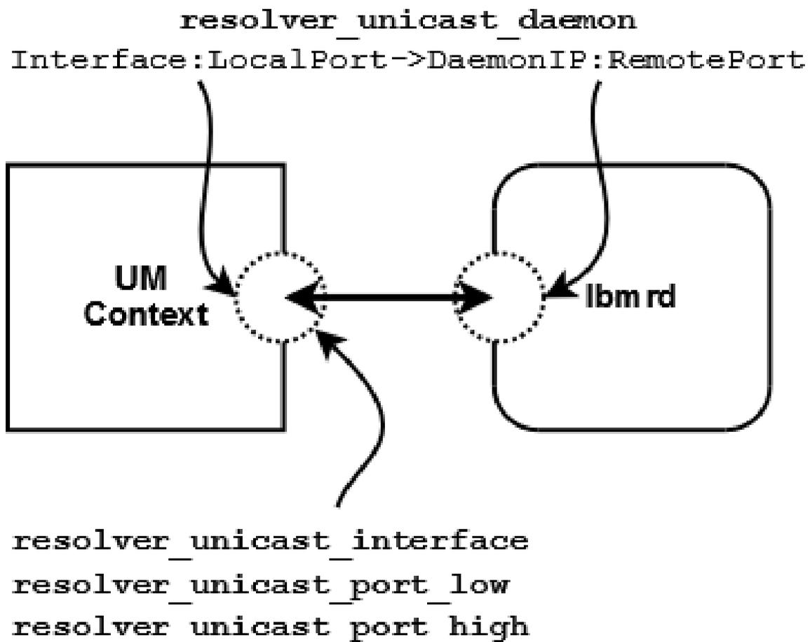
If using multiple `lbmrd` instances with a single context, you can configure `resolver_unicast_interface` and `resolver_unicast_port_low/high` and omit the `Interface:LocalPort` section of `resolver_unicast_daemon`.
